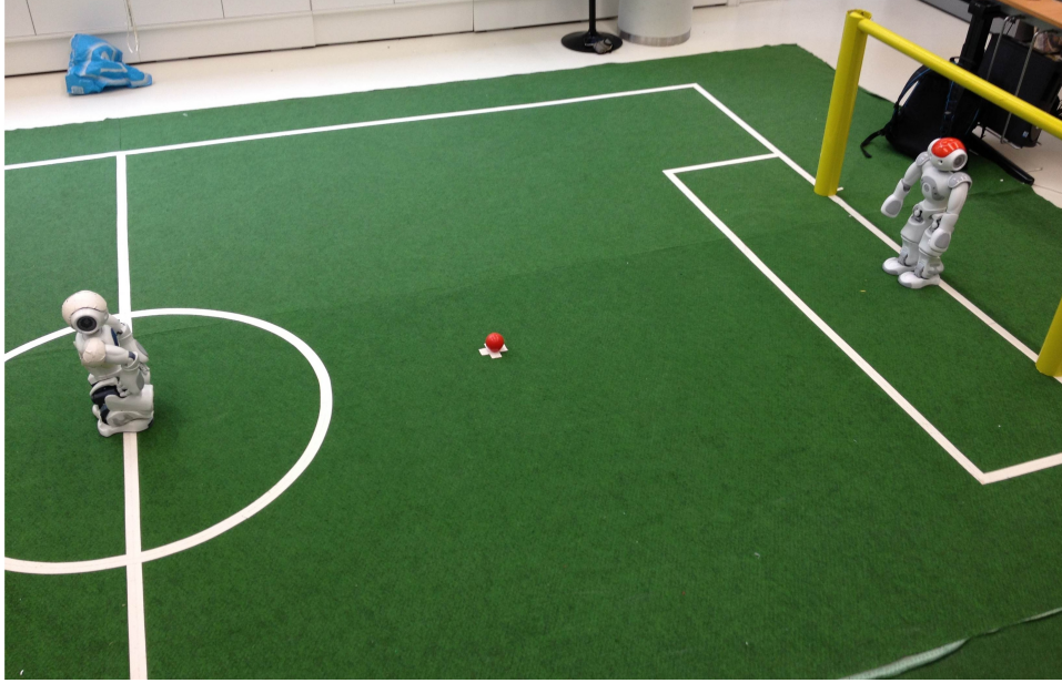
Figure 5: A typical start of a penalty shootout. The opposing player (left) starts at a distance of 3 meters to the goal, walks towards the ball, then kicks it.
