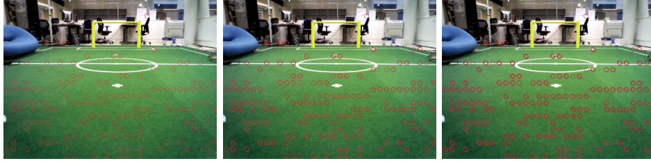
Figure 6: Three consecutive timesteps of a noisy motif z for N_z = 5 , T_z = 10 . Circles indicate cells where optical flow is found, with the thickness of the circle corresponding to presence p(w|z) . Obviously, this motif is too general to be of use.
